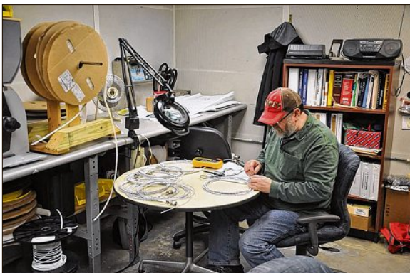
Dan Johnson, quality assurance technician, checks continuity and isolation of the wires in the wiring harness.
